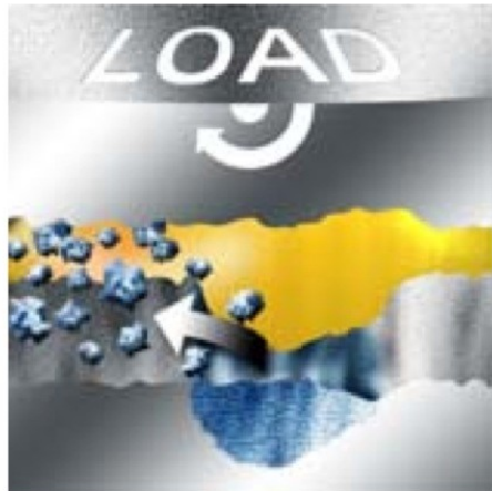
4. Surface fails + created particles
